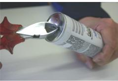
1. Remove rubber plug from base of aerosol can
