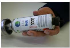
4. Screw canister including TUNAP Air Connector Adapter onto the TUNAP LPG Adapter until slight resistance is felt.
