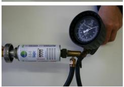
5. Connect air pressure gauge to Air Connector Adapter and apply a minimum of 8 bar pressure. Aerosol can empties within 5 seconds. Next finish air pressure application and remove air pressure gauge.
