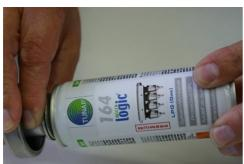
6. Hold TUNAP LPG Adapter with one hand and unscrew aerosol can.
