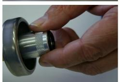
7. Unscrew TUNAP LPG Adapter from filler connector. Replace and screw protective cap onto filler connector and close fuel filler cover.
