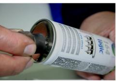
2. Screw TUNAP Air Connector Adapter (Product Code 11 1342) into the aperture in the base of the aerosol can.
