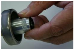
Open fuel filler cover and/or gas filler protective cap. Screw TUNAP LPG Adapter (Product Code 11 1340 or 11 1341) tightly onto the filler coupling. If necessary use commercially available intermediate adapter.
